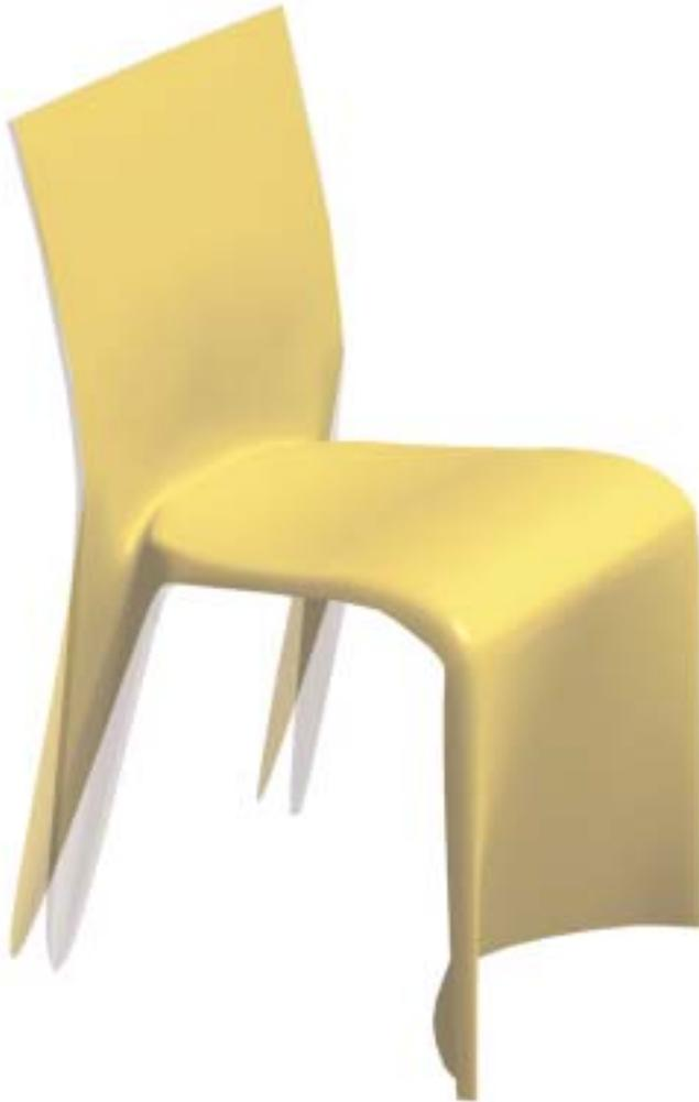
**Figure 11** Design 1:1, in which the rear legs are placed further back in an attempt to reduce the stress concentrations and undesired deformations.
