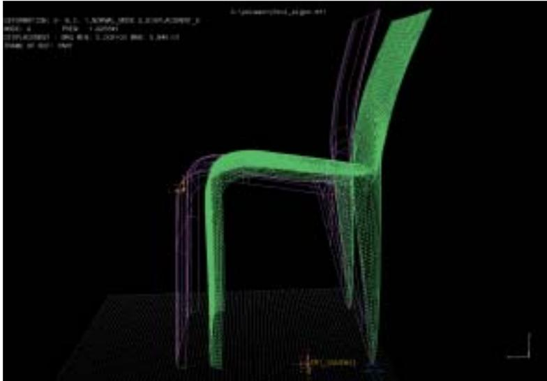
Figure 5 The second eigenmode of design 0.
