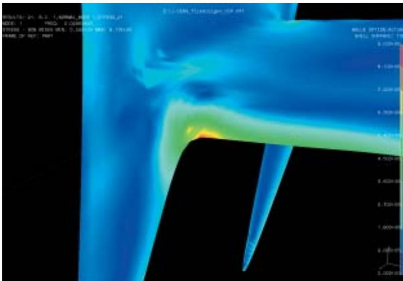
**Figure 10** The von Mises stresses associated with the first eigenmode. Detail: the joint between the seat, a rear leg and the backrest.
