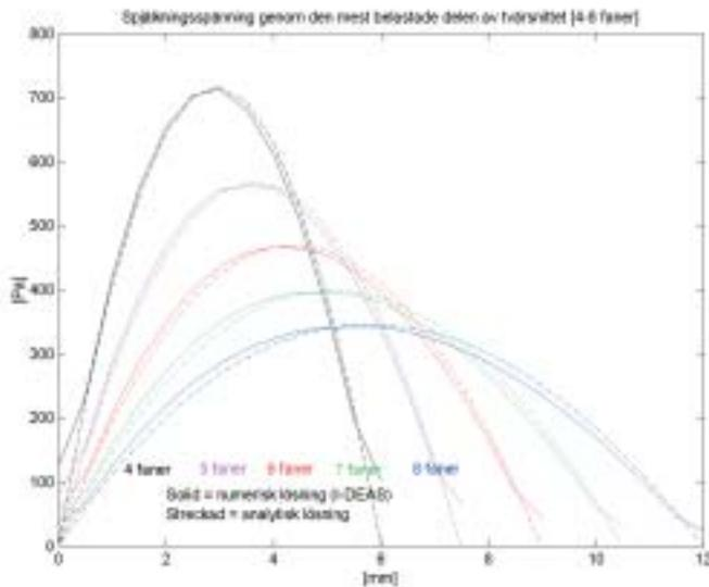
Figure 19 Delamination strains in laminates consisting of differing numbers of lamina.
