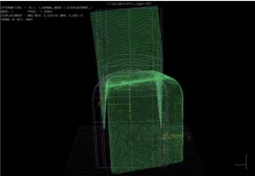
**Figure 4** The first eigenmode of design 0.
