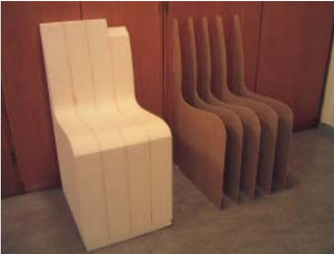
**Figure 2** A Styrofoam prototype used to test whether the chair in question is comfortable enough.
