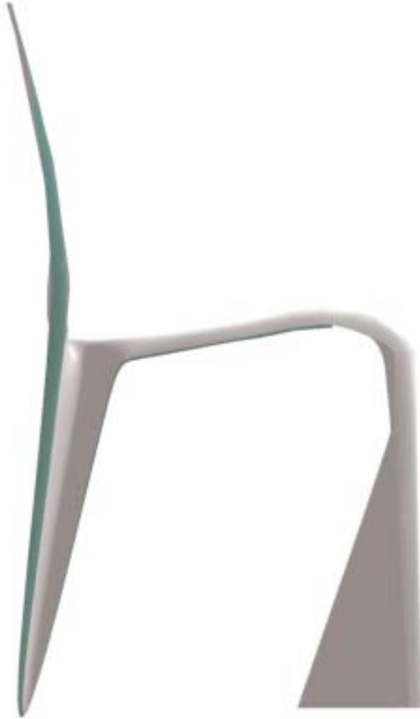
**Figure 13** Design 1:3, with a change in the profile of the leg and backrest, seen as another way of improving the chair's stability.
