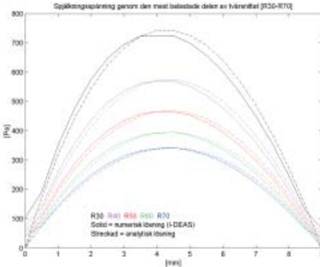
**Figure 20** Delamination strains in chair seats with differing radii of bending between the seat and the back of the chair.
